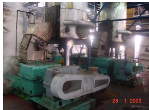
Screw press with digester above
